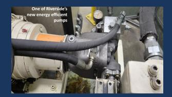
Luxfer Gas Cylinders in Riverside, CA has worked to reduce power consumption by replacing multiple pumps in their operations. These pumps rely on electric motors to power the equipment and to supply hydraulic pressure for hydrotesting Type 3 SCBA cylinders as part of the quality and product verification process. After considerable research, the Riverside team opted to install several new highefficiency pumps, which yield a 5.7 kWh reduction in power consumption.
