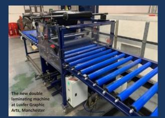
Luxfer Graphic Arts in Manchester, England has serviced the U.S., Japanese, and U.K. copper engraving market for many years. Engraving plates are traditionally laminated in lacquer to protect the back of the plate during the etching process. The Manchester team discovered the potential to substitute the lacquer with a laminate film. Following positive internal testing and keen interest from customers, the Manchester site installed a new double laminating machine.
