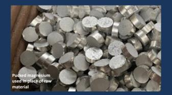
Luxfer Graphic Arts in Madison, IL creates magnesium rolled products. Magnesium sheets are flooded with mineral oil during the grinding process to keep the magnesium cool during processing and produce a smooth, high-quality finish. This process produces a mixed waste made of magnesium fines and mineral oil known as swarf.
